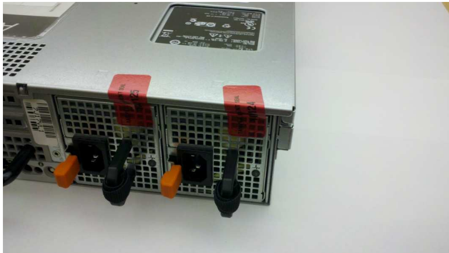
Figure 11 – Tamper-Evident Seal Application Positions (Power Supplies)
