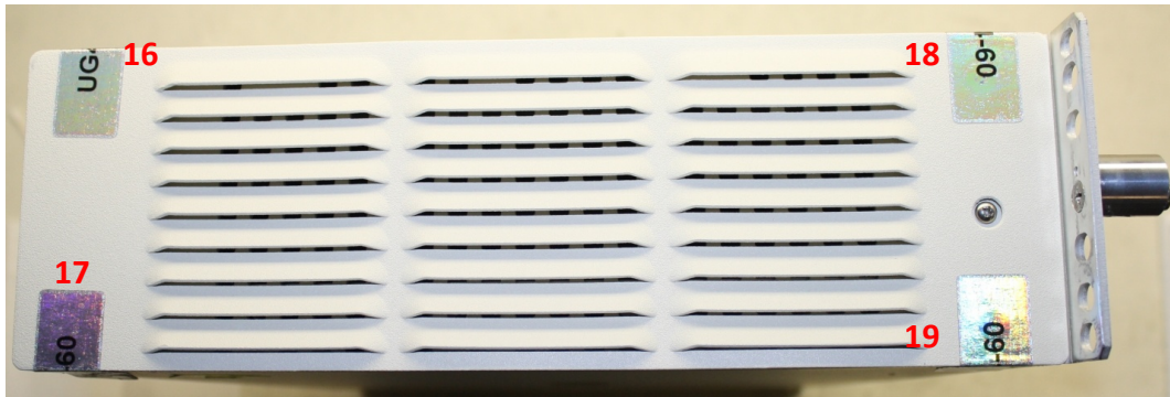
Figure 14 Location of Security Seals on Louver Panel (Left Side)
