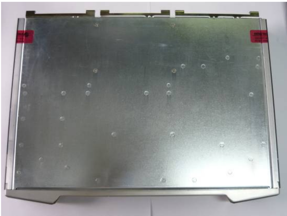
Figure 14 – Factory installed tamper seals
