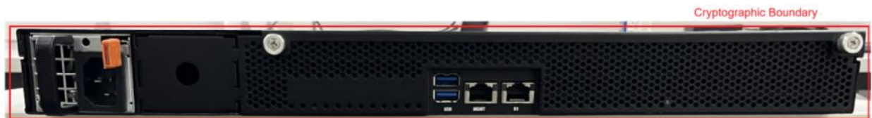
Figure 8: Rear Panel of the Trellix Intrusion Prevention System Sensor NS5200
