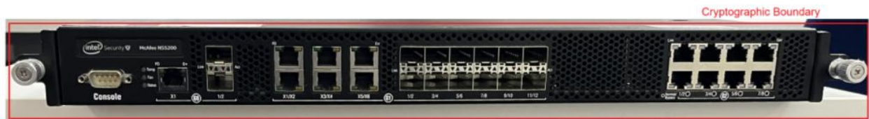
Figure 7: Front Panel of the Trellix Intrusion Prevention System Sensor NS5200
