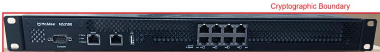
Figure 1: Front Panel of the Trellix Intrusion Prevention System Sensor NS3100
