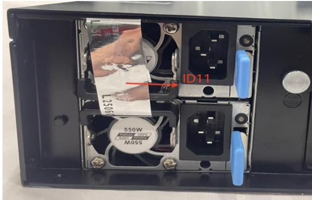
Figure 6 – Module A Seal Application Locations (Back)
