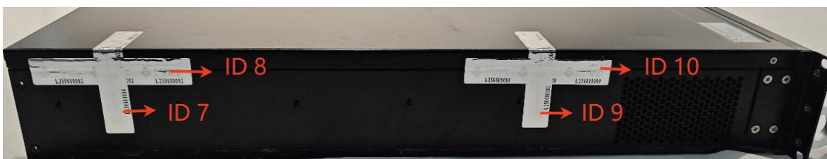
Figure 5 – Module A Seal Application Locations (Right side)
