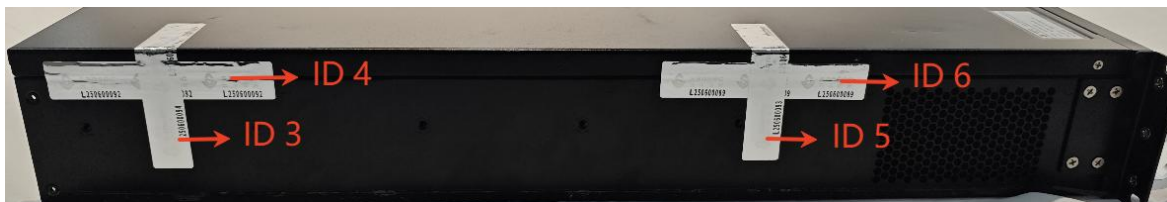
Figure 4– Module A Seal Application Locations (Left side)
