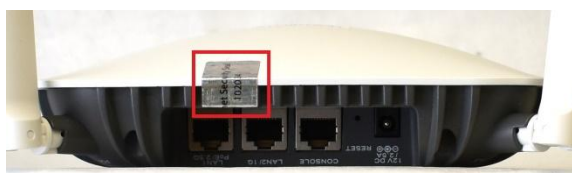
Figure 5 - FortiAP-233G seal placement.
