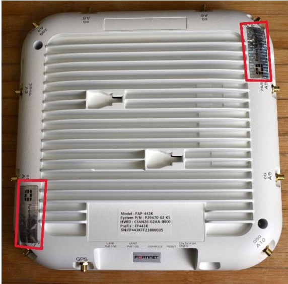
Figure 7 - FortiAP-443K seal placement.
