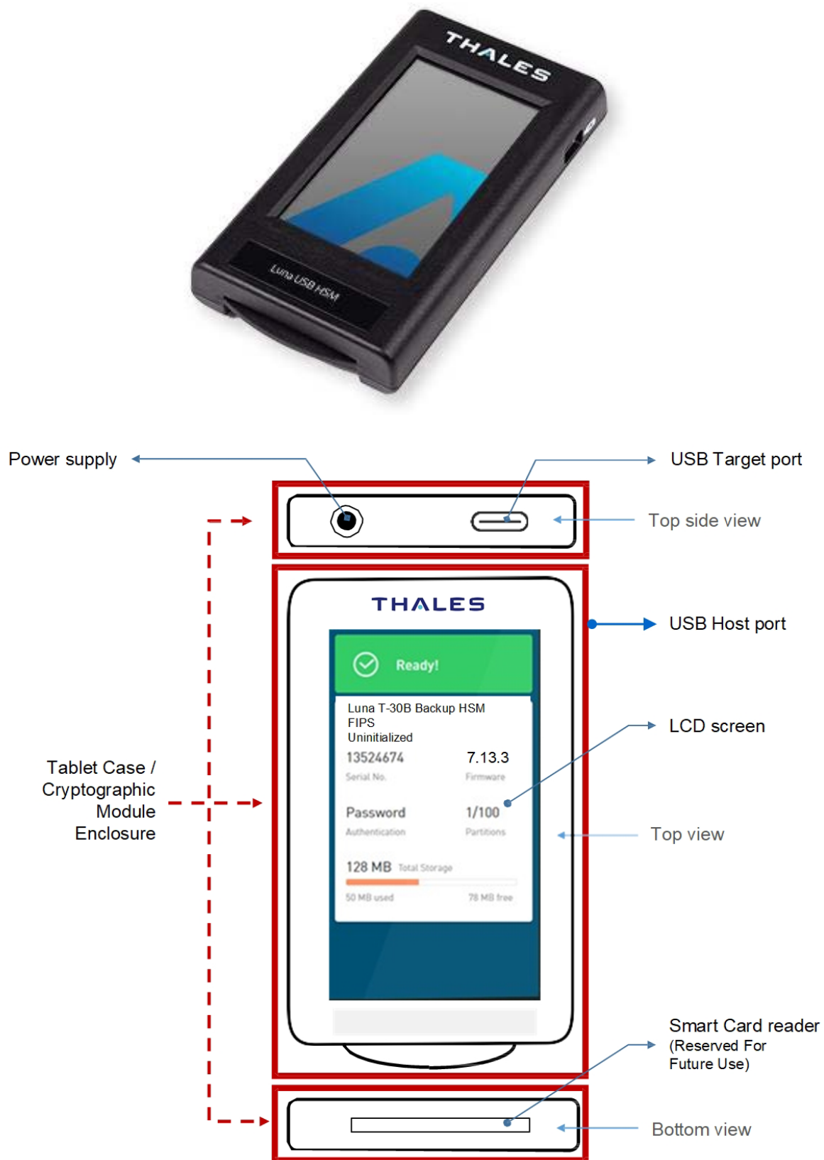
Figure 1: T-SERIES LUNA USB HSM Block Diagram, containing LUNA M7 Cryptographic Module, with external ports
