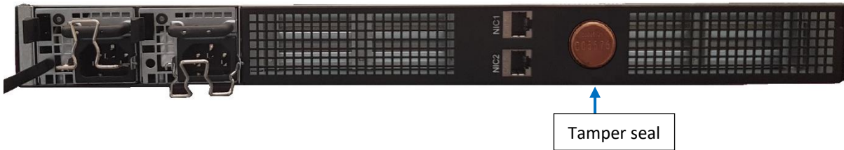
Figure 9 – QSCD Appliance Tamper Seal Location
