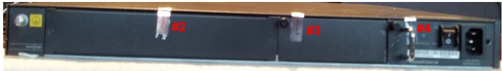
Figure 7-48: Tamper Seal Locations - Back
