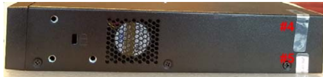
Figure 7-29: Tamper Seal Locations - Right Side
