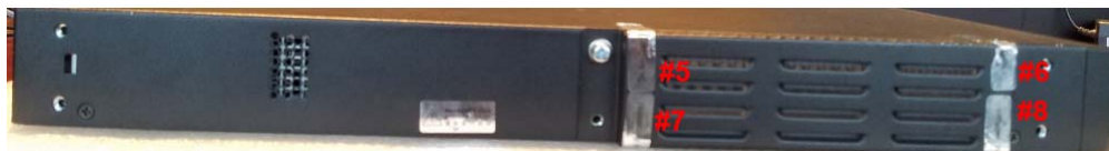
Figure 7-41: Tamper Seal Locations - Left Side Baffle
