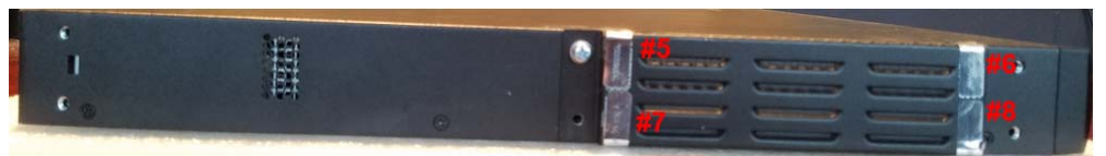
Figure 7-52: Tamper Seal Locations - Left Side Baffle
