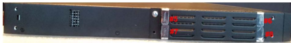
Figure 7-49: Tamper Seal Locations - Left Side Baffle
