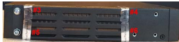
Figure 7-36: Tamper Seal Locations - Left Side Baffle
