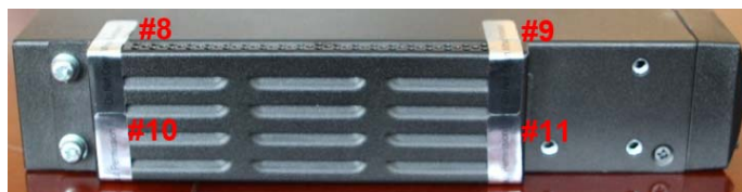
Figure 7-20: Tamper Seal Locations - Left Side Baffle
