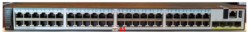
Figure 7-45: Tamper Seal Locations - Front
