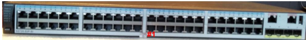
Figure 7-39: Tamper Seal Locations - Front
