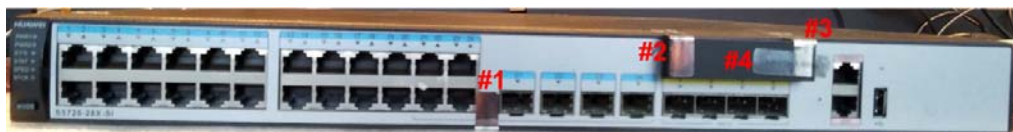
Figure 7-31: Tamper Seal Locations - Front
