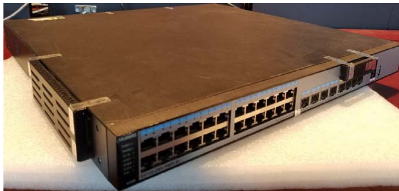
Figure 2-11: S5720-28X-PWR-SI-AC (Top, Left, Front)
