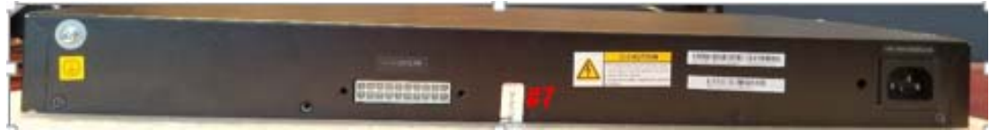
Figure 7-19: Tamper Seal Locations - Back
