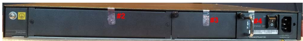
Figure 7-51: Tamper Seal Locations - Back
