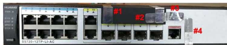
Figure 7-8: Tamper Seal Locations - Front
