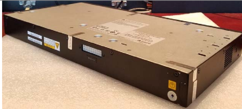
Figure 2-14: S5720-28X-SI-24S-AC (Bottom, Right, Back)
