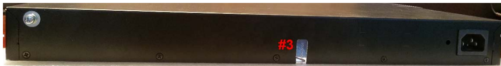
Figure 7-22: Tamper Seal Locations - Back
