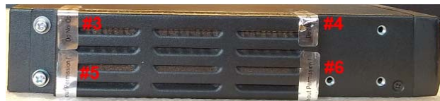
Figure 7-44: Tamper Seal Locations - Left Side Baffle
