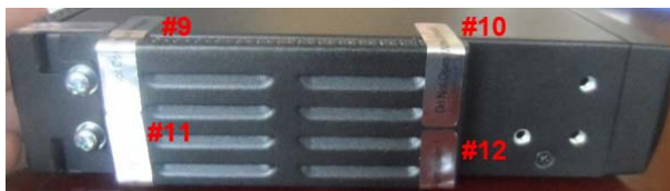
Figure 7-10: Tamper Seal Locations - Left Side Baffle
