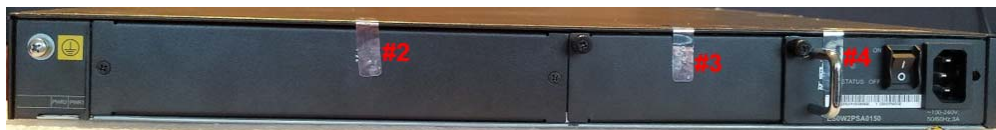
Figure 7-40: Tamper Seal Locations - Back
