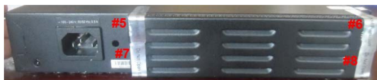
Figure 7-9: Tamper Seal Locations – Back Baffle
