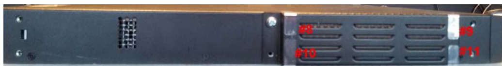
Figure 7-26: Tamper Seal Locations - Left Side Baffle
