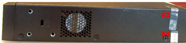
Figure 7-16: Tamper Seal Locations - Right Side
