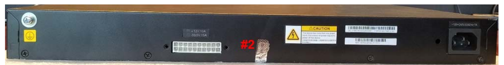
Figure 7-46: Tamper Seal Locations - Back
