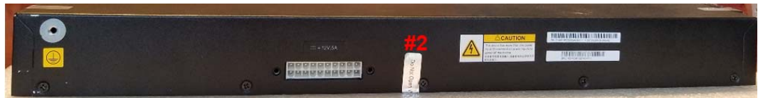
Figure 7-15: Tamper Seal Locations - Back
