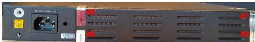
Figure 7-12: Tamper Seal Locations – Back Baffle
