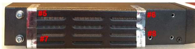
Figure 7-17: Tamper Seal Locations - Left Side Baffle
