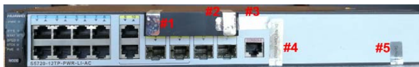
Figure 7-11: Tamper Seal Locations - Front
