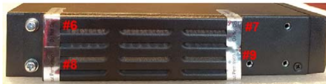
Figure 7-30: Tamper Seal Locations - Left Side Baffle
