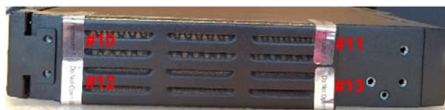
Figure 7-13: Tamper Seal Locations - Left Side Baffle
