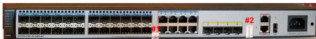
Figure 7-27: Tamper Seal Locations - Front
