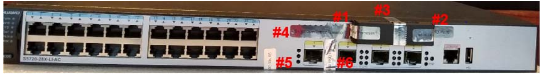
Figure 7-18: Tamper Seal Locations - Front
