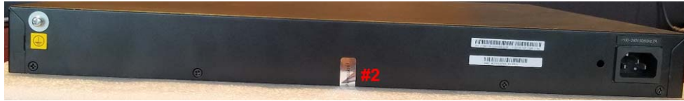
Figure 7-38: Tamper Seal Locations - Back
