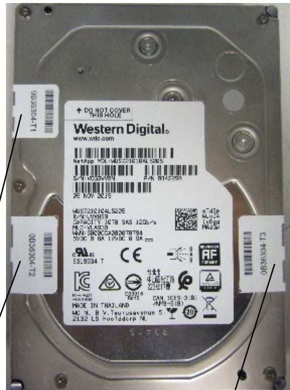
Figure 5: Wrapping Tamper-Evident Seals
