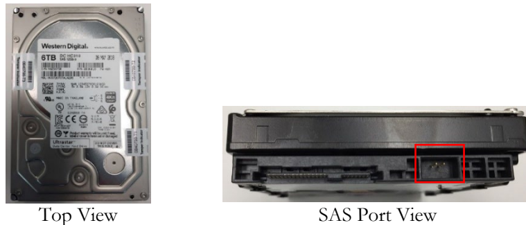
Figure 2: Cryptographic Boundary for Ultrastar DC HC320
