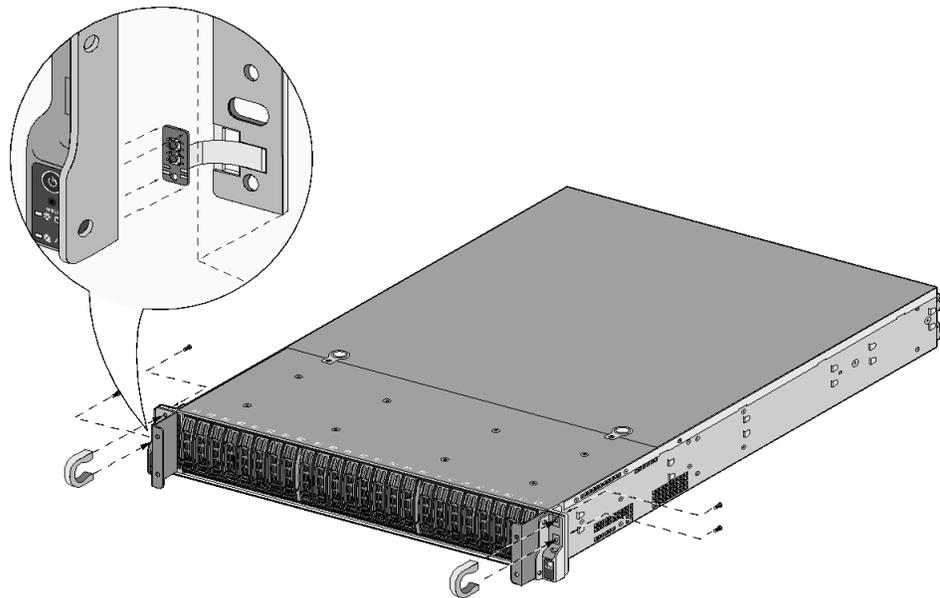
Figure 10 - Attach Pull Handles and Front Modules
