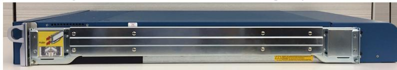
Figure 4 - Right side of WF-500 with opacity shields
