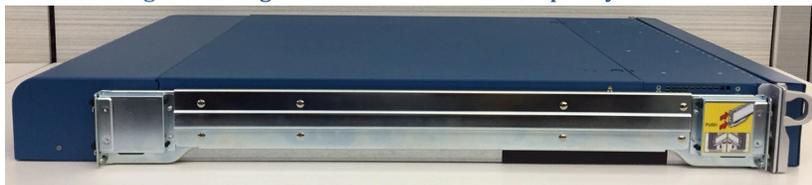
Figure 5 - Left side of WF-500 with opacity shields
