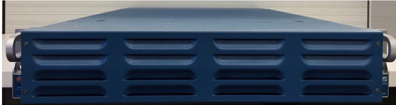
Figure 2 - Front view of WF-500 with opacity shield
