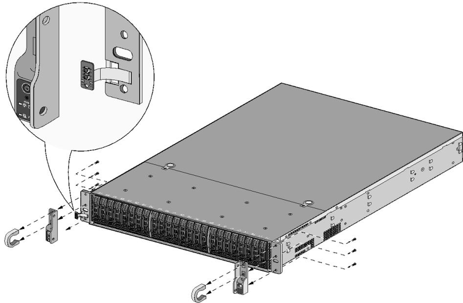
Figure 8 - Remove Front Handles and Modules
