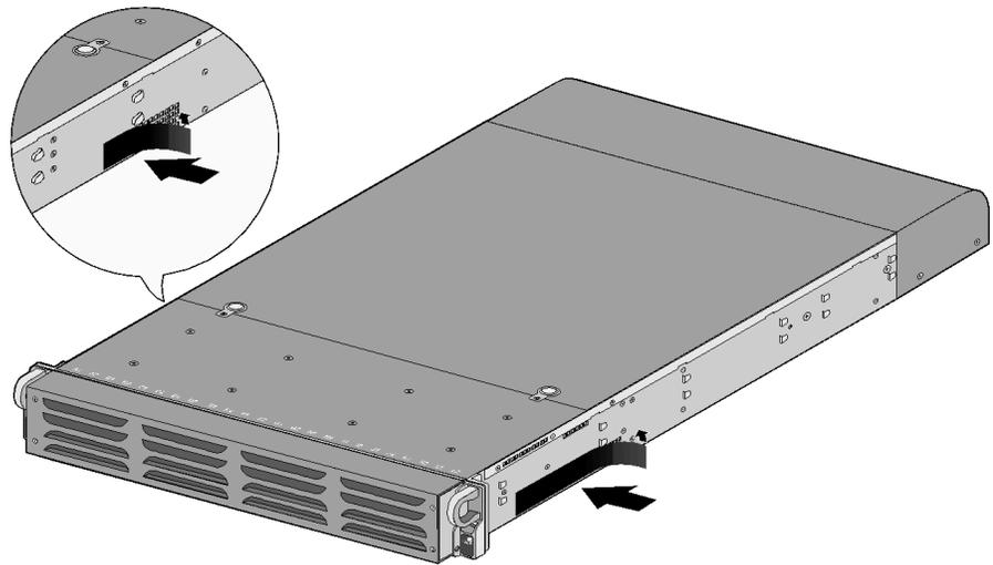
Figure 15 - Apply Tamper-Evident Seals on Vent Overlays
