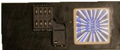
Figure 3. SecureD FPGA Sample (front) – Epoxy Coated with Tamper Sticker Sample
