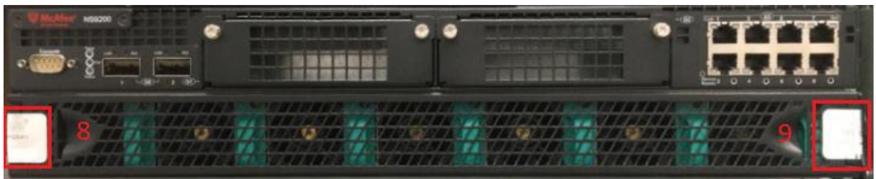
Figure 7 – Tamper Label Placement Front (9300 S)
