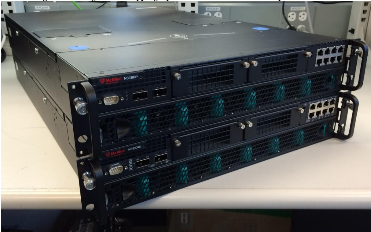
Figure 2 – Image of the Cryptographic Module connected to its peer NS-9300 P
