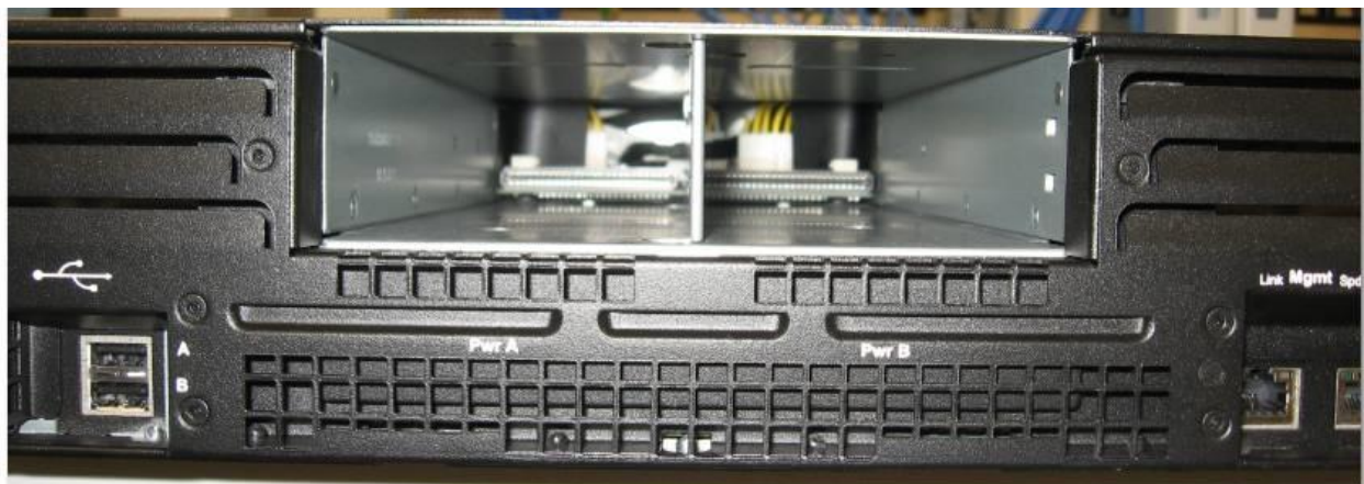
Figure 5 - Rear Panel with Power Supplies Removed
