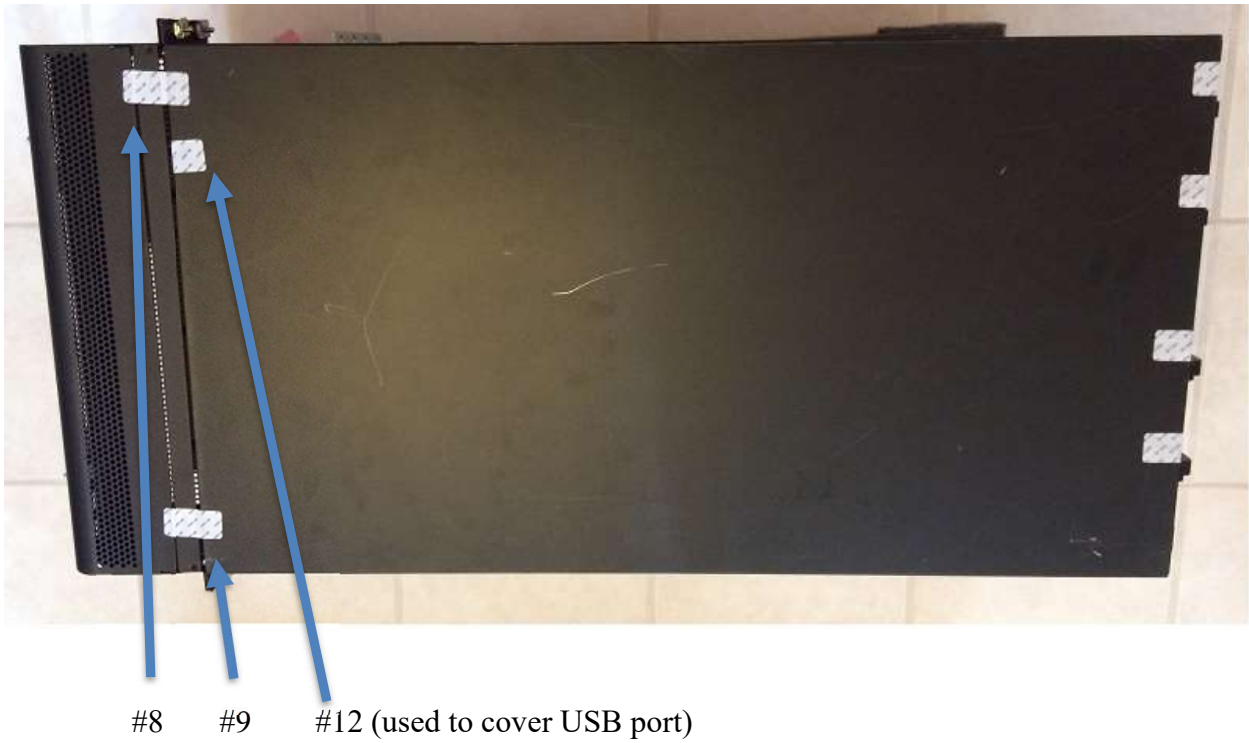
Figure 11: Top 9300 Series (Top has TEL #8 and #9 overlapping opacity shield and top of chassis, also present is TEL #3, #4, #5, #6 and #7. TEL #12 partially obscured inside the opacity shield, overlapping front of chassis and top of chassis covering the USB)
