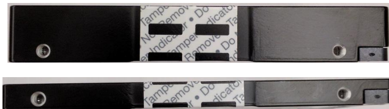
Figure 5: Right-side view of tamper-evidence label on right side of Nytro 3000® SAS Interface module
