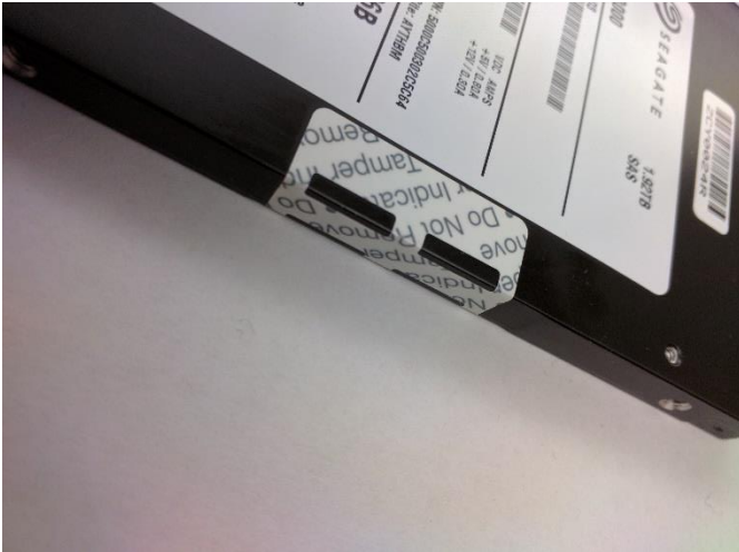
Figure 6: Nytro 3000® 7mm Top Cover Tamper Evidence
