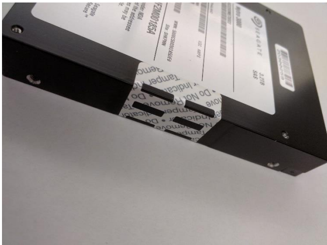
Figure 8: Nytro 3000® 15mm Top Cover Tamper Evidence
