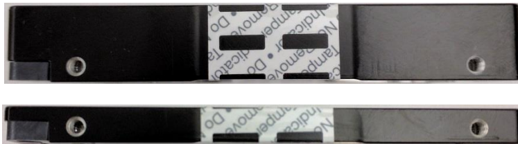
Figure 4: Left-side view of tamper-evidence label on left side Nytro 3000® SAS Interface module
