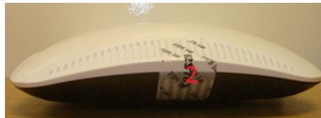
Figure 11 – Right Side View of AP-204 / AP-205 with TELs
