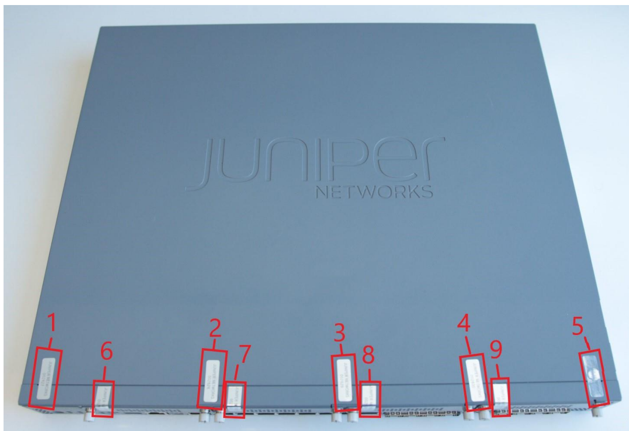
Figure 22 - SRX340/SRX345 Tamper-Evident Seal Placement (Top Cover, Nine (9) Seals: TEL 1-5; Across covering vertically the front I/O Slots, Four Seals: TEL 6-9)
