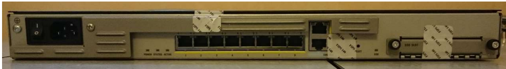
Figure 36 ASA 5516-X Rear TEL Placement
