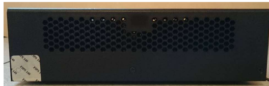
Figure 22 ASA 5506H-X Right Side TEL Placement
