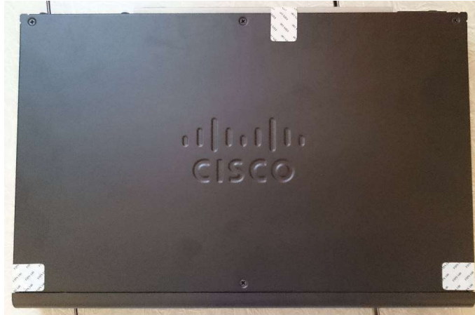
Figure 31 ASA 5508-X Top TEL Placement
