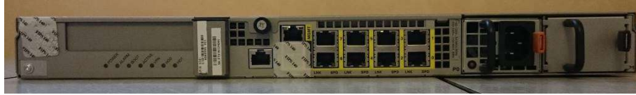
Figure 54 ASA 5555-X Rear TEL Placement
