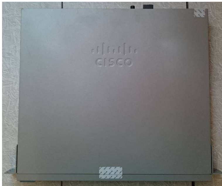
Figure 43 ASA 5525-X Top TEL Placement
