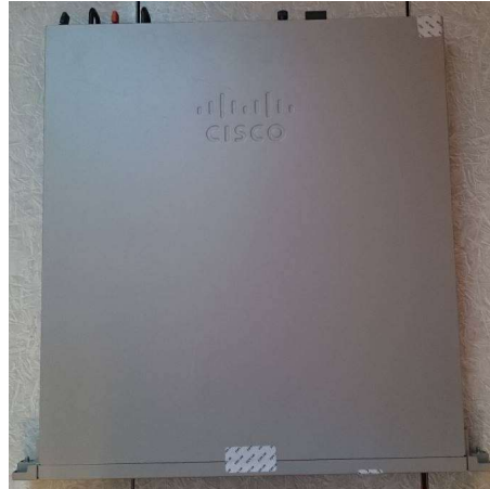
Figure 55 ASA 5555-X Top TEL Placement
