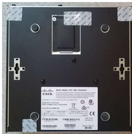
Figure 26 ASA 5506H-X Bottom TEL Placement
