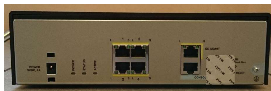
Figure 24 ASA 5506H-X Rear TEL Placement
