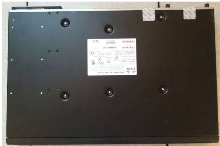
Figure 32 ASA 5508-X Bottom TEL Placement
