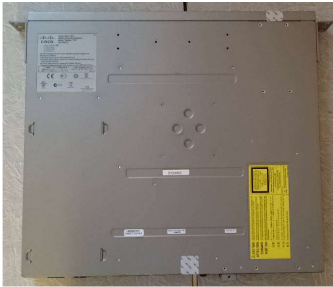
Figure 44 ASA 5525-X Bottom TEL Placement
