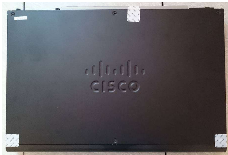
Figure 37 ASA 5516-X Top TEL Placement
