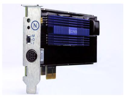
The following figure shows the nCipher nShield cryptographic module:
