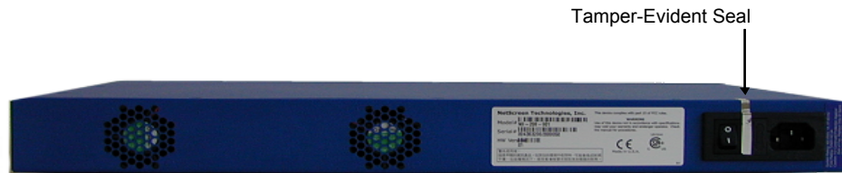
Figure 3: Tamper evident seal on AC interface
