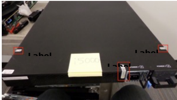
Figure 10 - BIG-IP i5000 (3 of 3 tamper labels)
