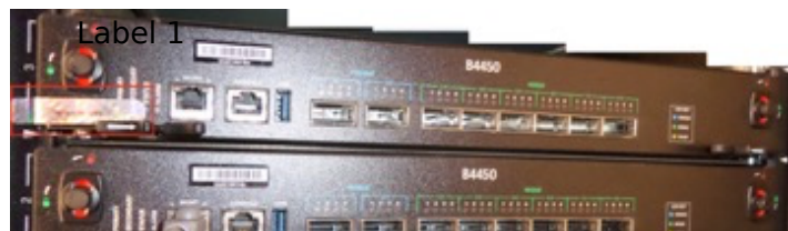
Figure 17 - VIPRION B4450 front (1 of 5 tamper labels shown)
