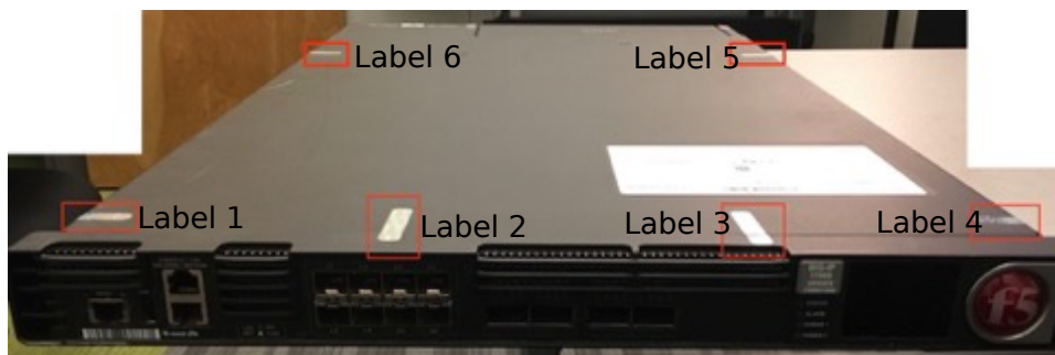
Figure 11 - BIG-IP i5820-DF (4 of 4 tamper labels shown)
