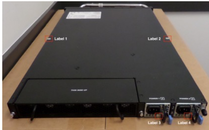
Figure 11 - BIG-IP i5820-DF (4 of 4 tamper labels shown)
