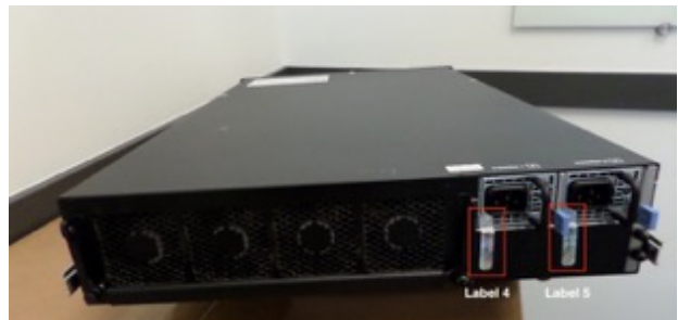
Figure 15 - BIG-IP i15800 (Back tamper labels 4 and 5 labels shown)
