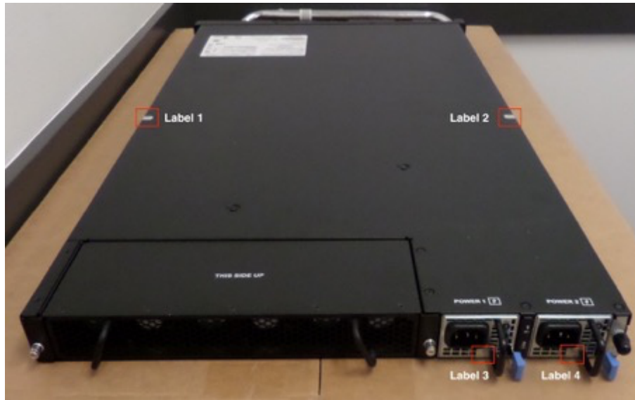
Figure 13 - BIG-IP i7820-DF (4 of 4 tamper labels shown)
