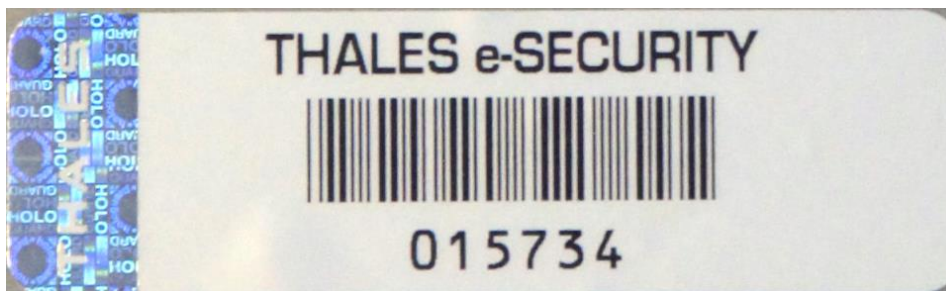
Figure 3: Close-up of Thales tamper-evident label
