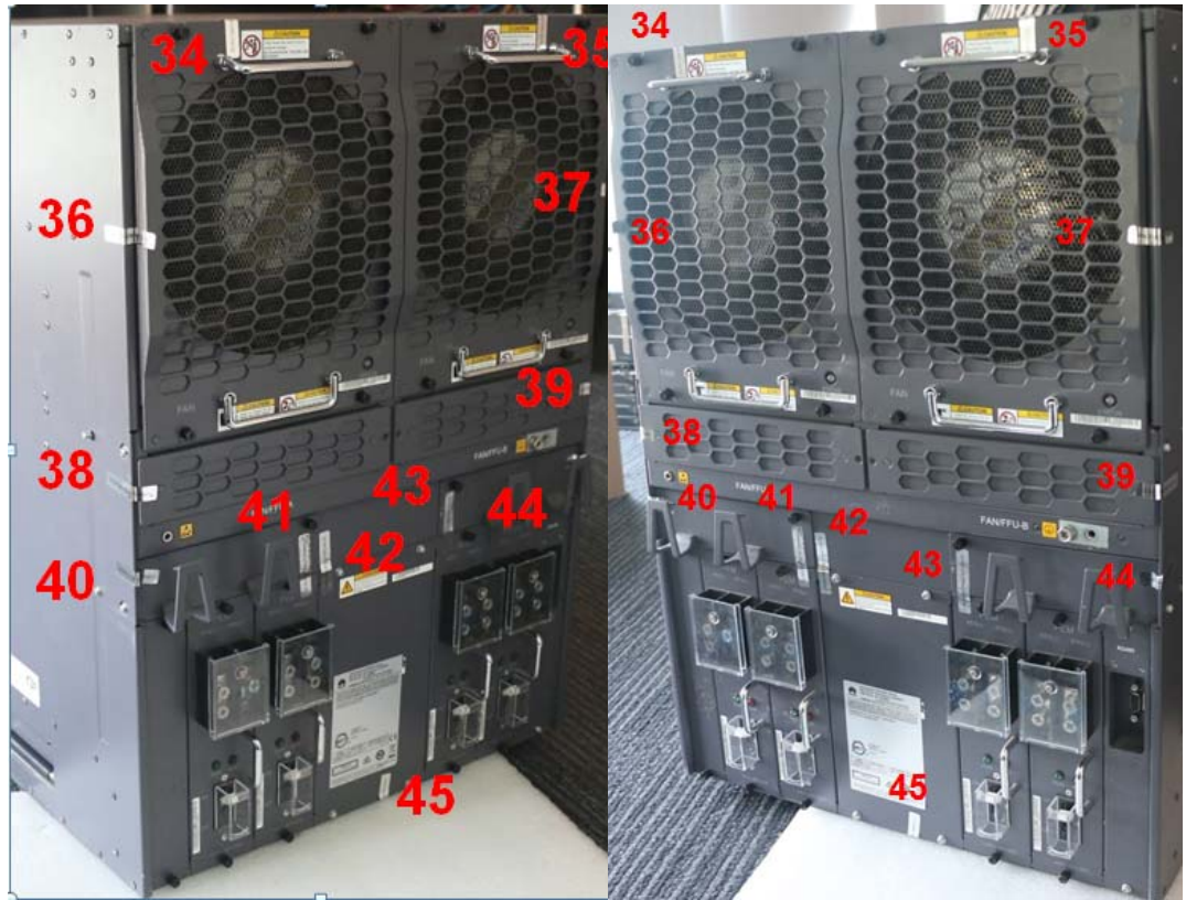
Figure 6-11 USG9560 Tamper Seal Placement- Back, Left and Right Sides
