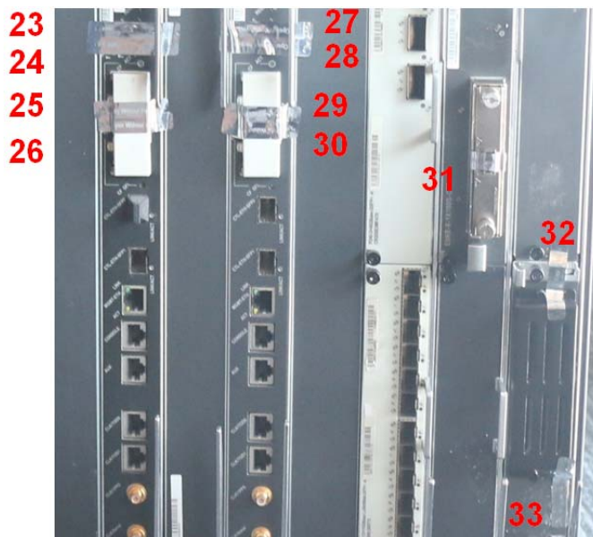
Figure 6-10 USG9560 Tamper Seal Placement- Front Middle
