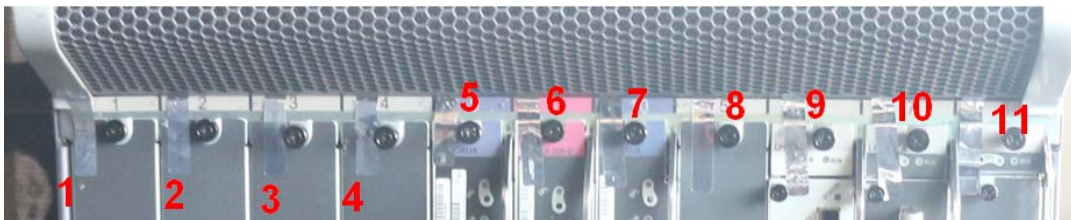
Figure 6-8 USG9560 Tamper Seal Placement- Front Top
