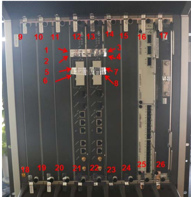
Figure 6-13 USG9580 Tamper Seal Placement- Upper Half of Front
