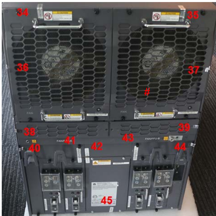
Figure 6-12 USG9560 Tamper Seal Placement- Back and Top
