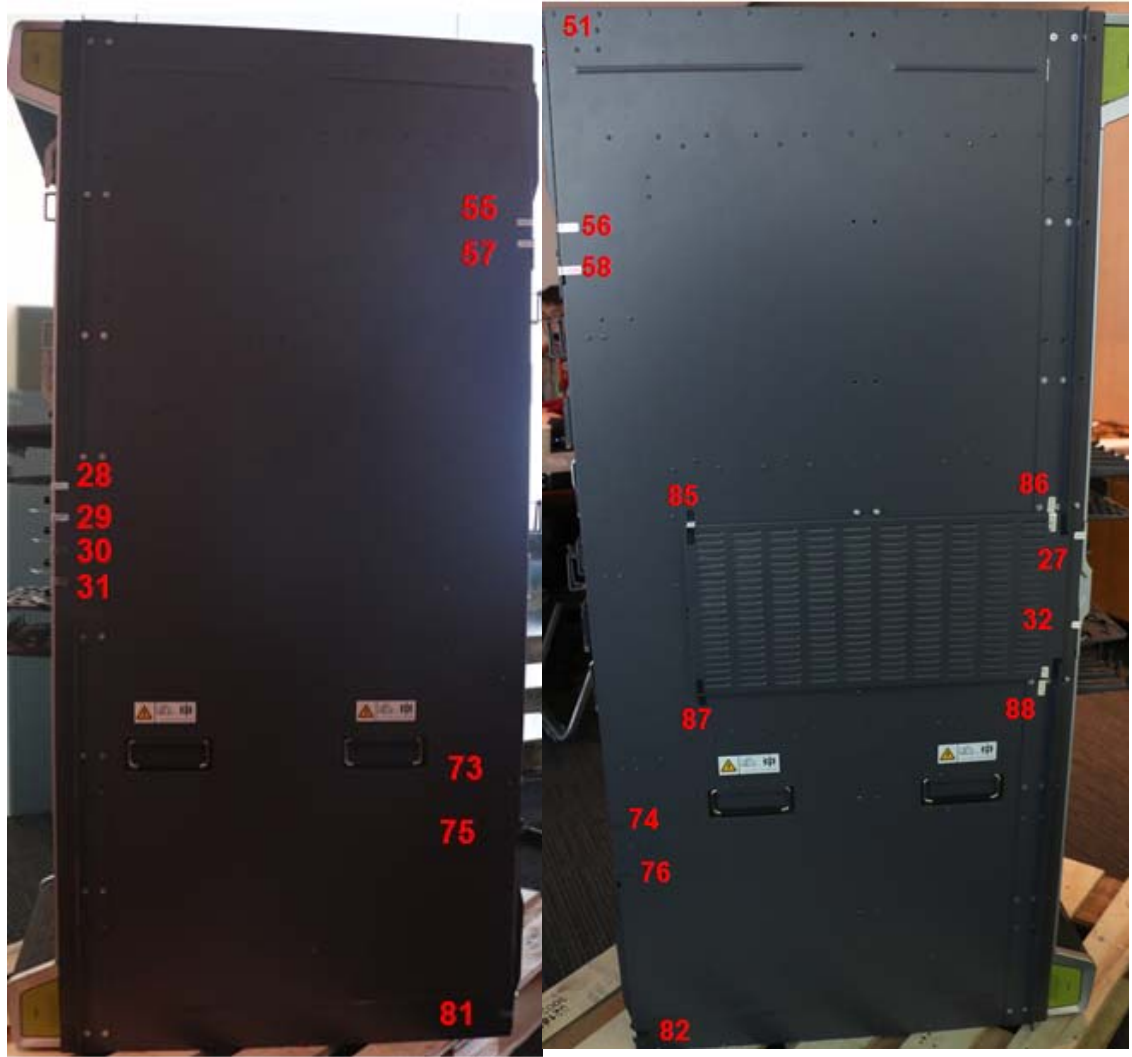
Figure 6-16 USG9580 Tamper Seal Placement- Right and Left Sides
