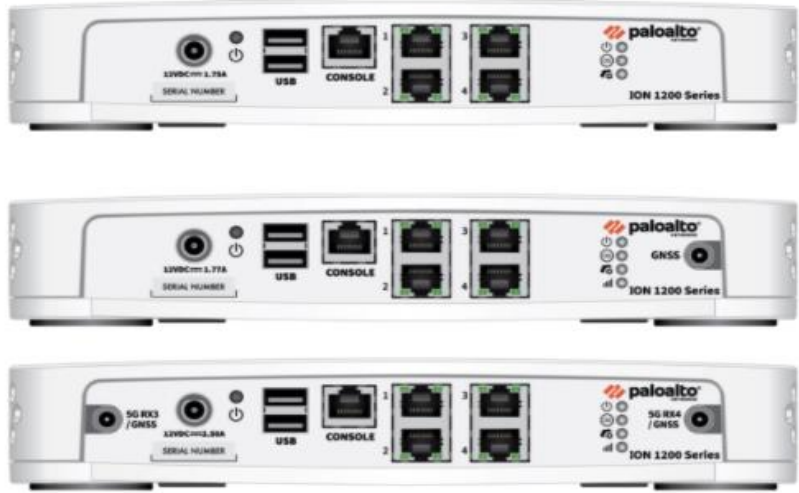
Figure 3 - ION 1200 (Top), ION 1200-C-NA/ION 1200-C-ROW (Middle), and ION 1200-C-5G-WW (Bottom) Front Interfaces
