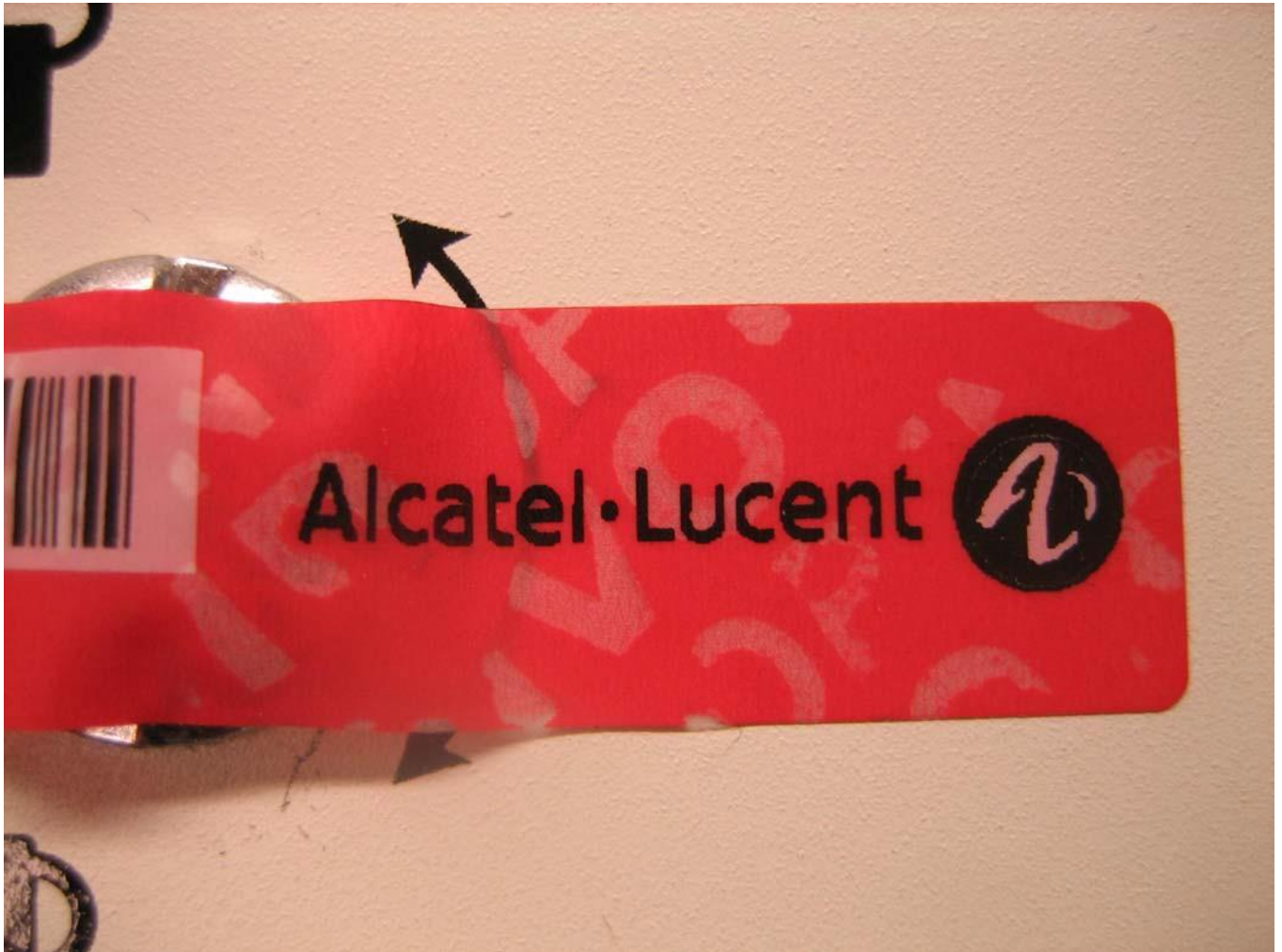
Figure 10 Tamper-evident label: broken (close-up view)
