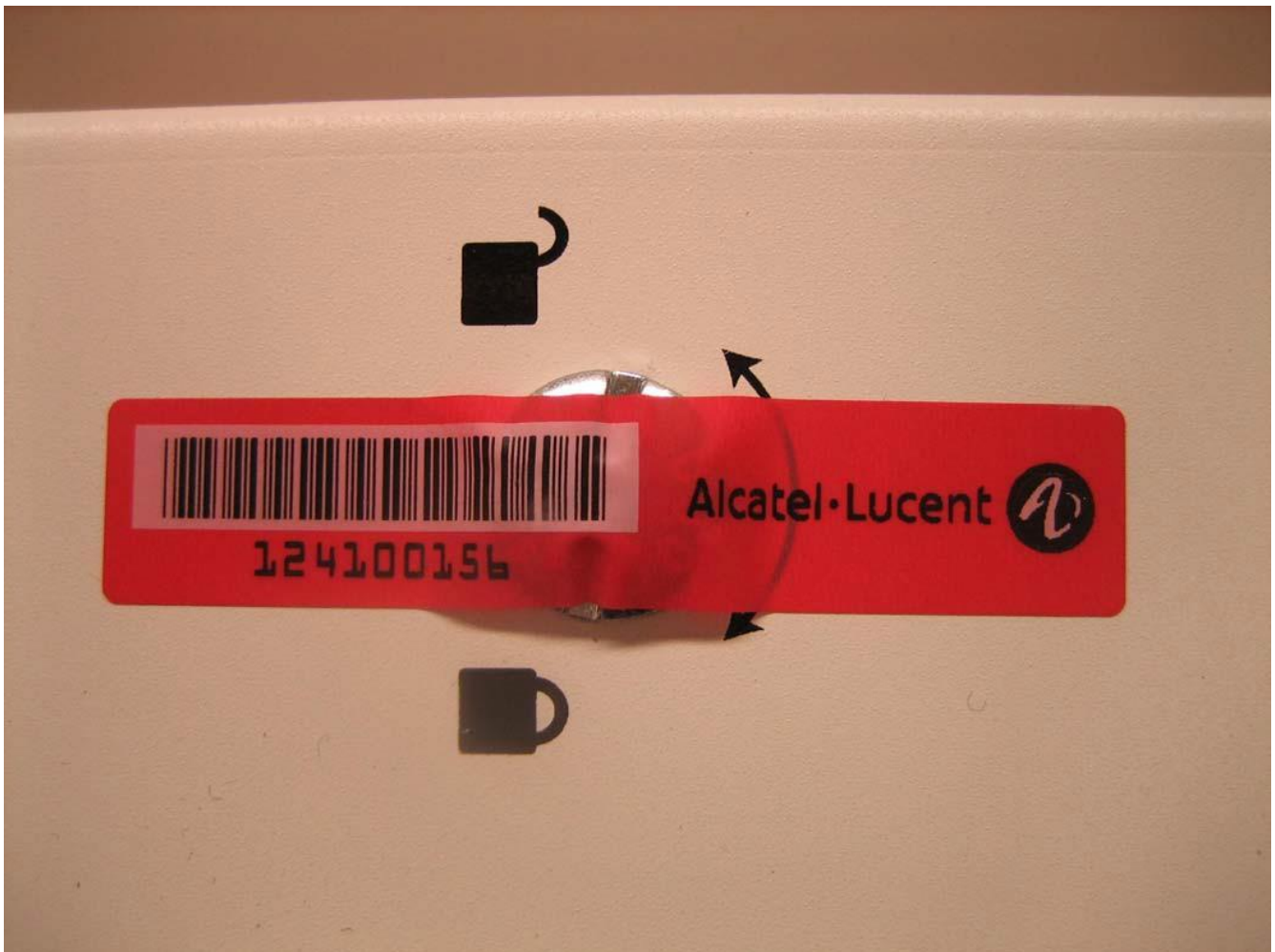
Figure 8 Tamper-evident label: intact
