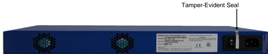
Figure 3: Tamper evident seal on AC interface
