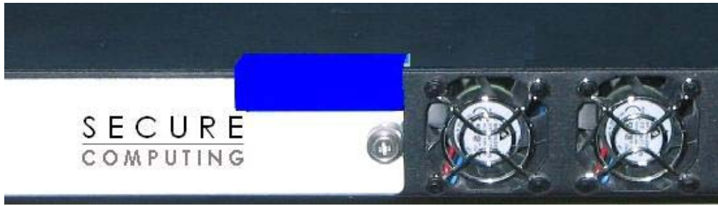
Figure 7 – Apply label to upper hard drive bay of the rear of the 500
