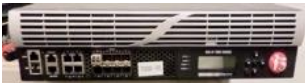
Figure 26 – BIG-IP 7000 with faceplate attached (Label 1 is located under faceplate)
