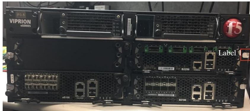
Figure 35 – VIPRION B2250 in chassis (1 of 6 tamper labels shown)
