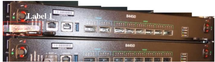
Figure 38 – VIPRION B4450 front (1 of 5 tamper labels shown)
