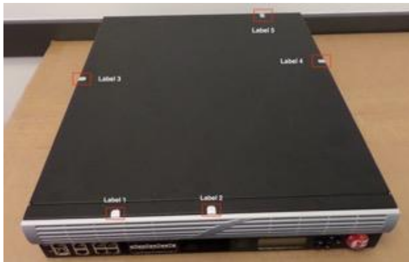
Figure 29 – BIG-IP 7200v-F (5 tamper labels shown)
