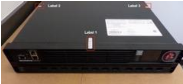
Figure 22 – BIG-IP i15800 (Front tamper labels 1-3 labels shown)
