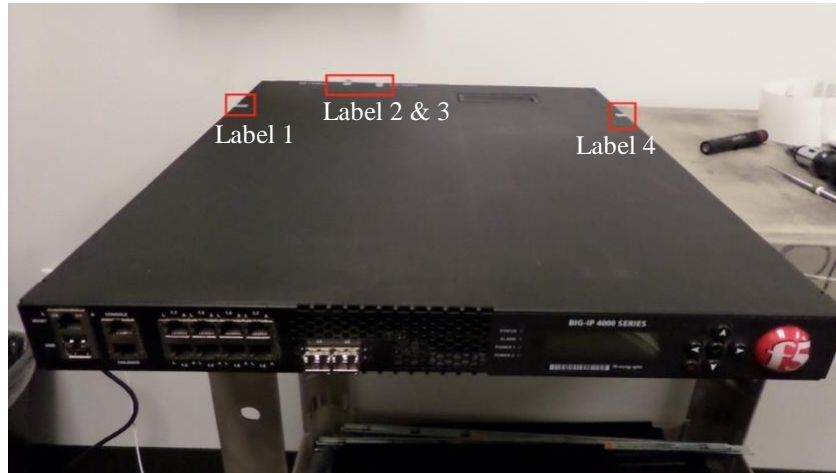
Figure 24 – BIG-IP 4000 (3 tamper labels shown)
