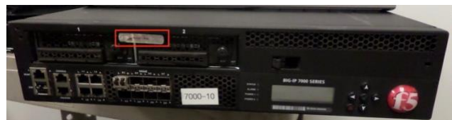
Figure 27 – BIG-IP 7000 with faceplate removed (1 of 4 tamper labels shown)
