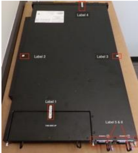
Figure 20 – BIG-IP i10800/i11800-DS (6 tamper labels shown)
