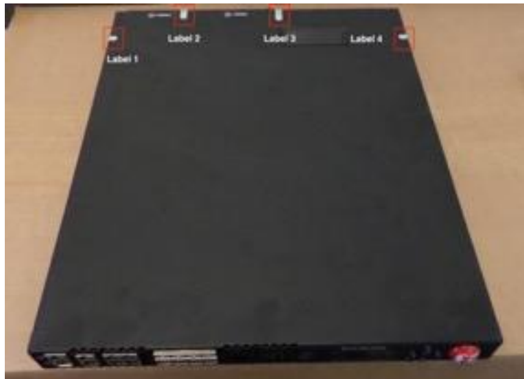
Figure 25 – BIG-IP 5250v-F (4 tamper labels shown)
