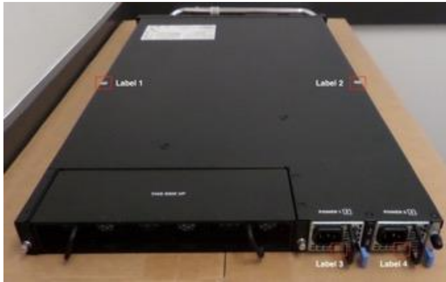
Figure 19 – BIG-IP i7820-DF (4 tamper labels shown)
