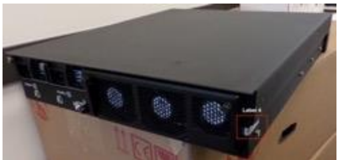
Figure 31 – BIG-IP 10200v-F (tamper label 4 shown)
