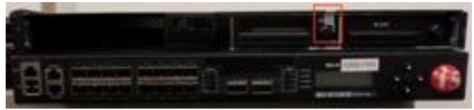
Figure 33 – BIG-IP 10350v-F with faceplate removed (1 of 4 tamper labels shown)
