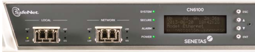
Figure 15 – A6100B 10G Ethernet port close-up - XFPs installed
