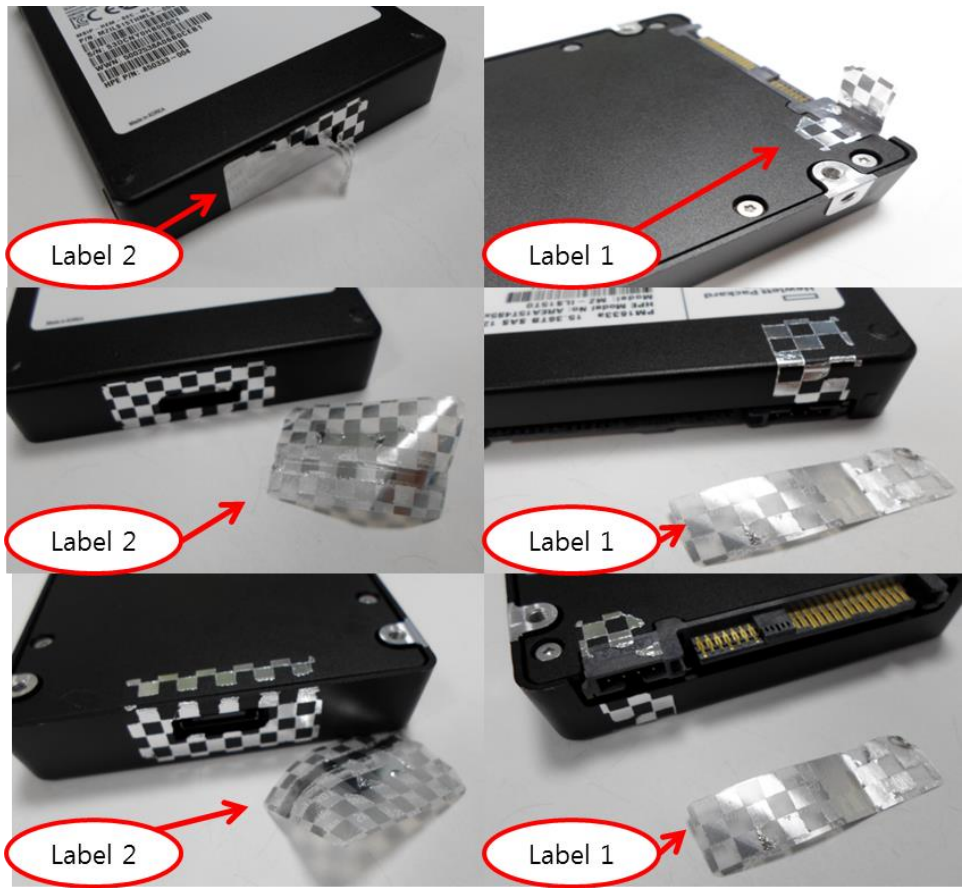
Exhibit 16 – Signs of Tamper
