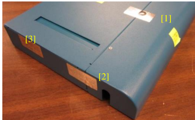
Figure 30 - PA-200 Left Side and Top Tamper Seal Placement (3)
