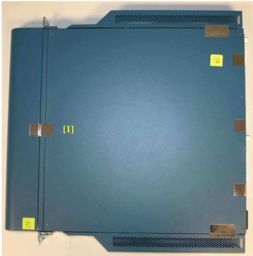
Figure 36 - PA-2000 Series Front Tamper Seal Placement (1)
