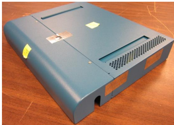
Figure 3 - PA-200 with Front Opacity Shield and Cage Enclosure
