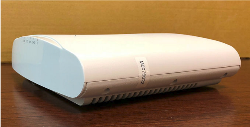
Figure 11: Tamper-evident seals on R720 Access Point
