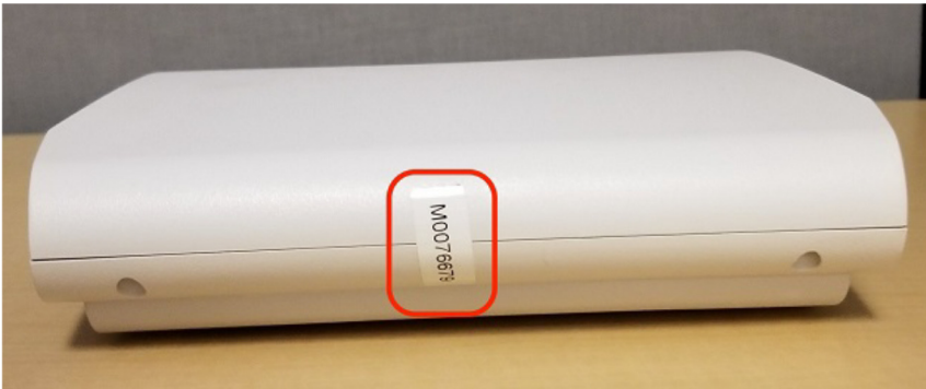
Figure 10: Tamper-evident seals on R710 Access Point
