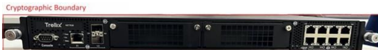
Figure 1: Front Panel of the Trellix Intrusion Prevention System Sensor NS7500
