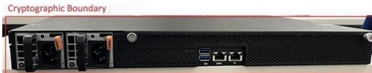
Figure 2: Rear Panel of the Trellix Intrusion Prevention System Sensor NS7500
