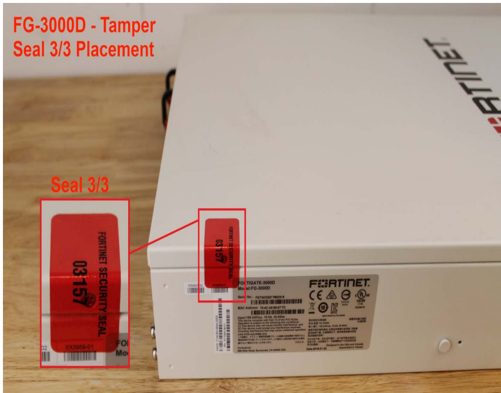
Figure 19 - FortiGate-3000D external enclosure seal, top, left side
