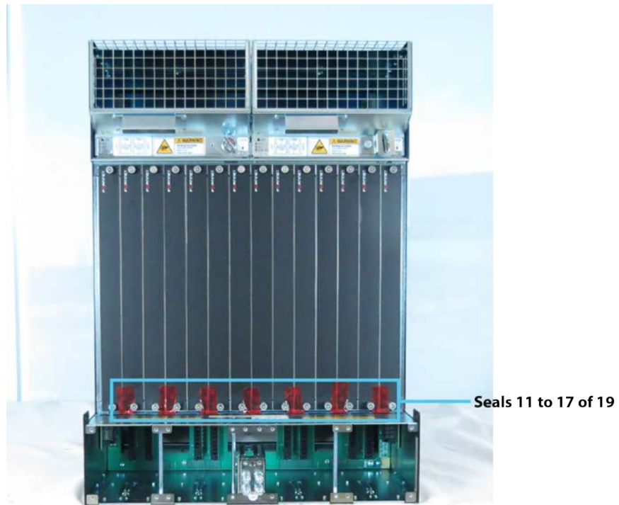
Figure 13 - FortiGate-5001D seals, rear view
