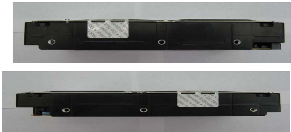
Figure 5: Constellation® ES.3 (SAS/SATA Interface) security labels on sides of drive
