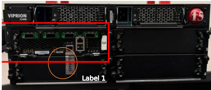
Figure 14 - Tamper labels on chassis with VIPRION B2250 blade (delineated by a red box) and three blanks (1 of 1 tamper label shown)
