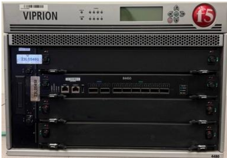
Figure 7 - B4450 blade mounted in VIPRION chassis 4480 with three blanks
