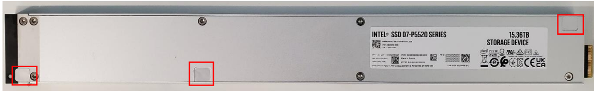
Figure 7 - E1.L Module (Intel Branded) Seal Application Locations – Bottom
