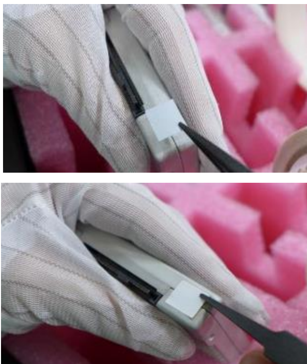
Figure 8 - Applying Tamper-Evident Seals
