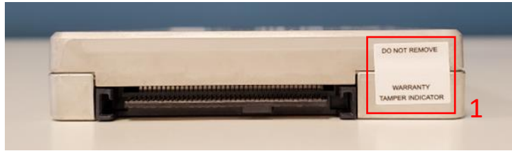
Figure 6 - U.2 Module Seal Application Locations - Front
