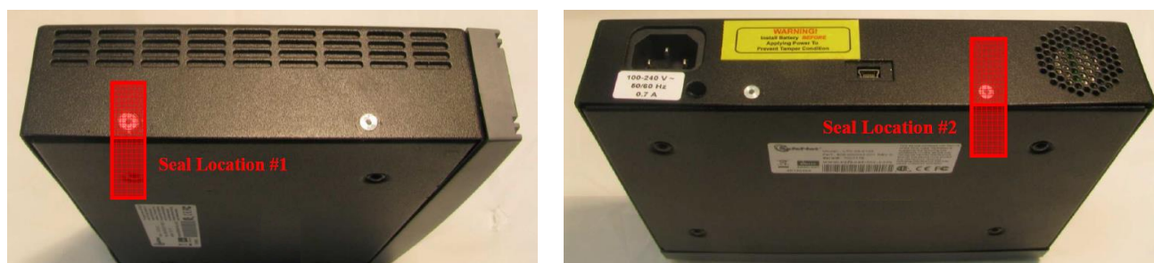
Figure 3-1. Tamper Evident Label Locations
