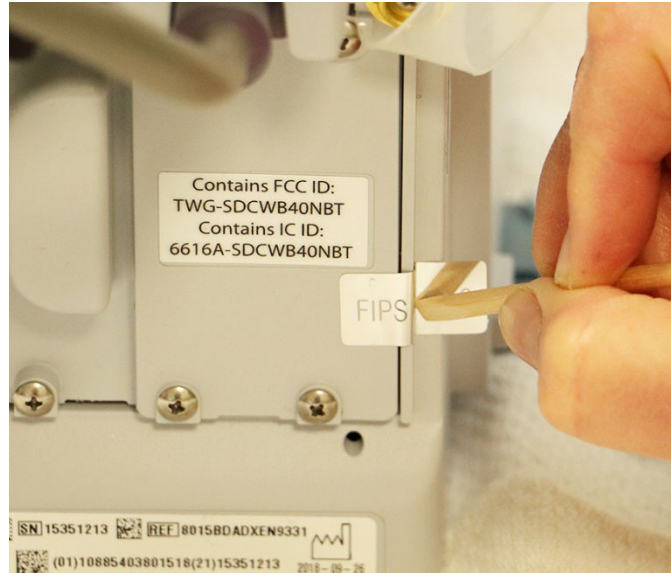
Figure 9–4: Using Orange Stick to Ensure Seal is Affixed
