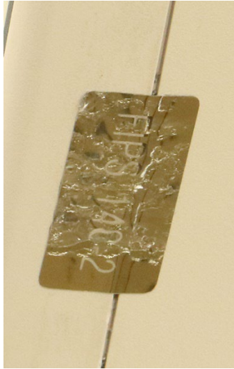
Figure 9-23: Tampered FIPS Seal
