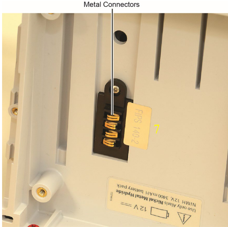
Figure 9-16: FIPS S on Battery Connector
