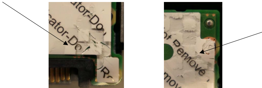
Figure 3: Tamper Evidence on Tamper Seal
