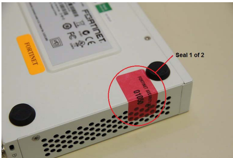
Figure 3: FortiWiFi-60C external enclosure seal, bottom, right side
