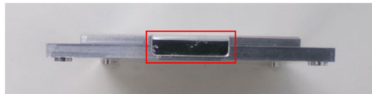
Figure 5: Location of Tamper Seal #2 (Bottom Edge)
