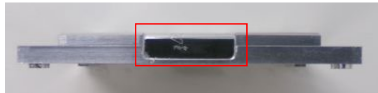
Figure 4: Location of Tamper Seal #1 (Top Edge)
