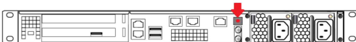
Figure 11-2: Thales Luna Network HSM decommission button location
