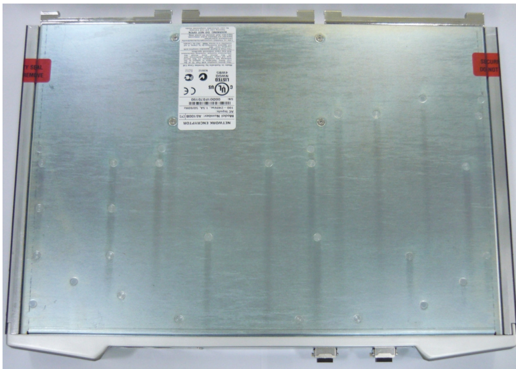
Figure 16 – Factory installed tamper seals
