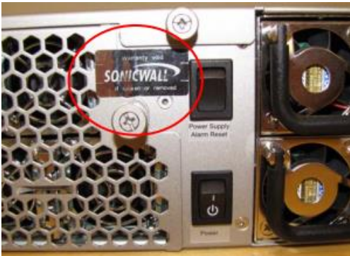
Figure 4 – EX-9000 Tamper Seal #5 - Rear Fans
