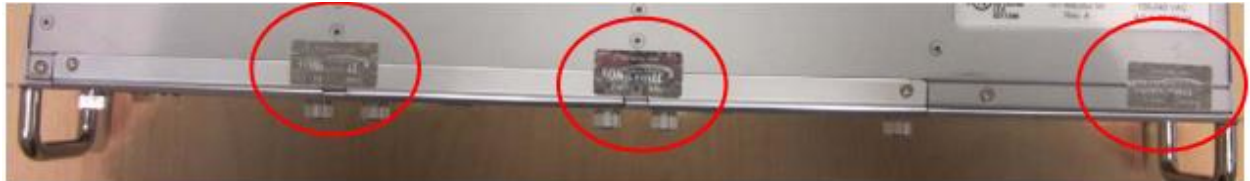
Figure 3 –EX-9000 Underside Tamper Seals #2, #3 and #4
