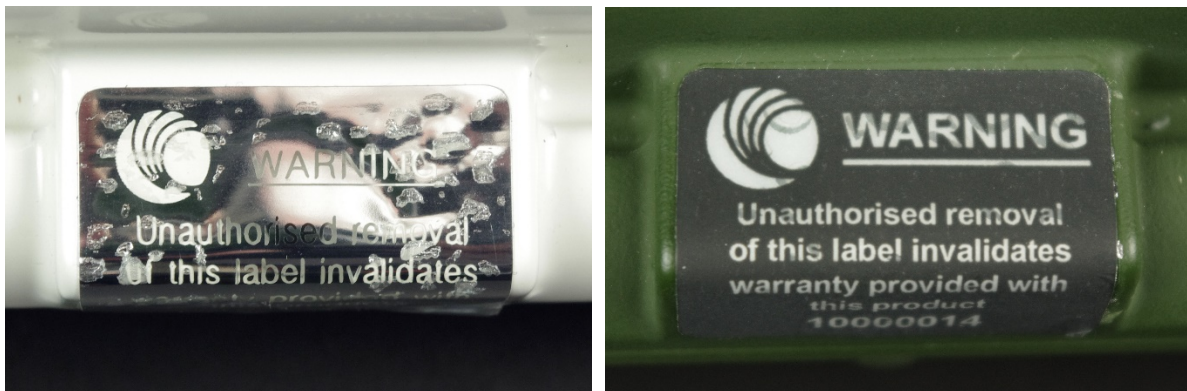
Figure 16 - Example of Tampered Seals
