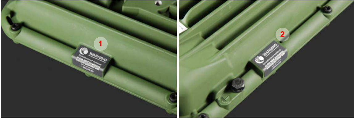
Figure 14 - Tamper-Evident Seal Locations on a Green Connectorized PTP 45700 Unit
