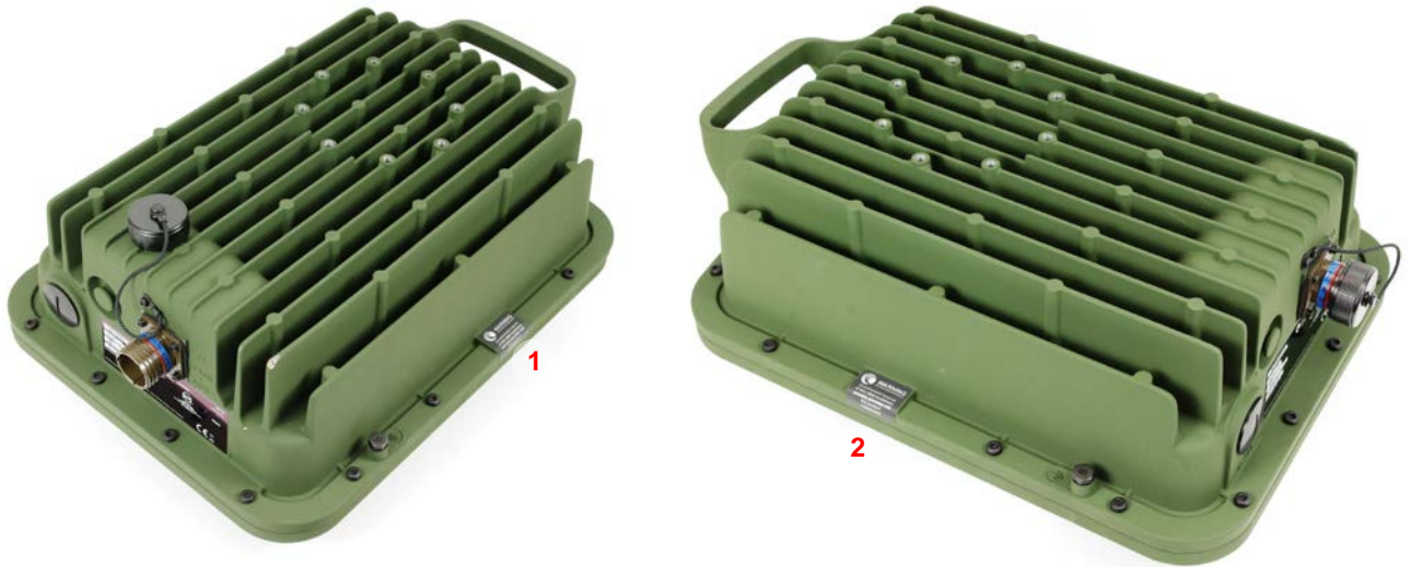
Figure 15 - Tamper-Evident Seal Locations on a PTP 78700 Unit
