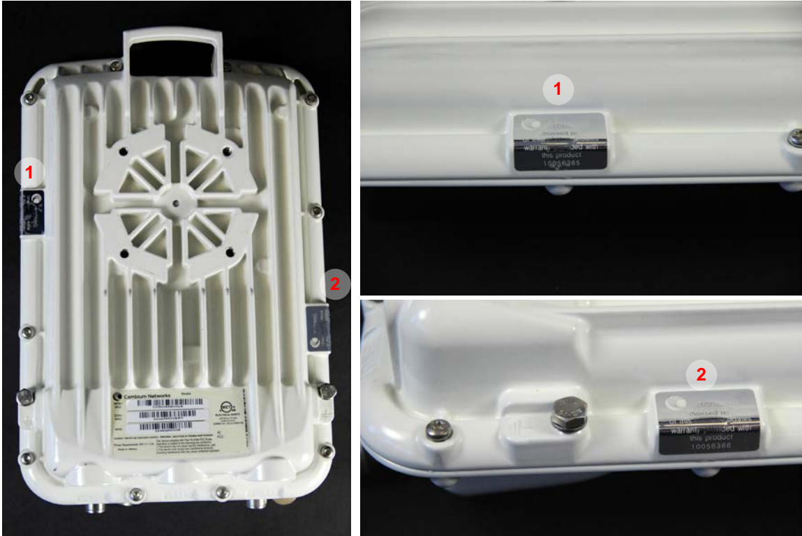
Figure 12 - Tamper-Evident Seal Locations on a White Connectorized PTP 45700 Unit
