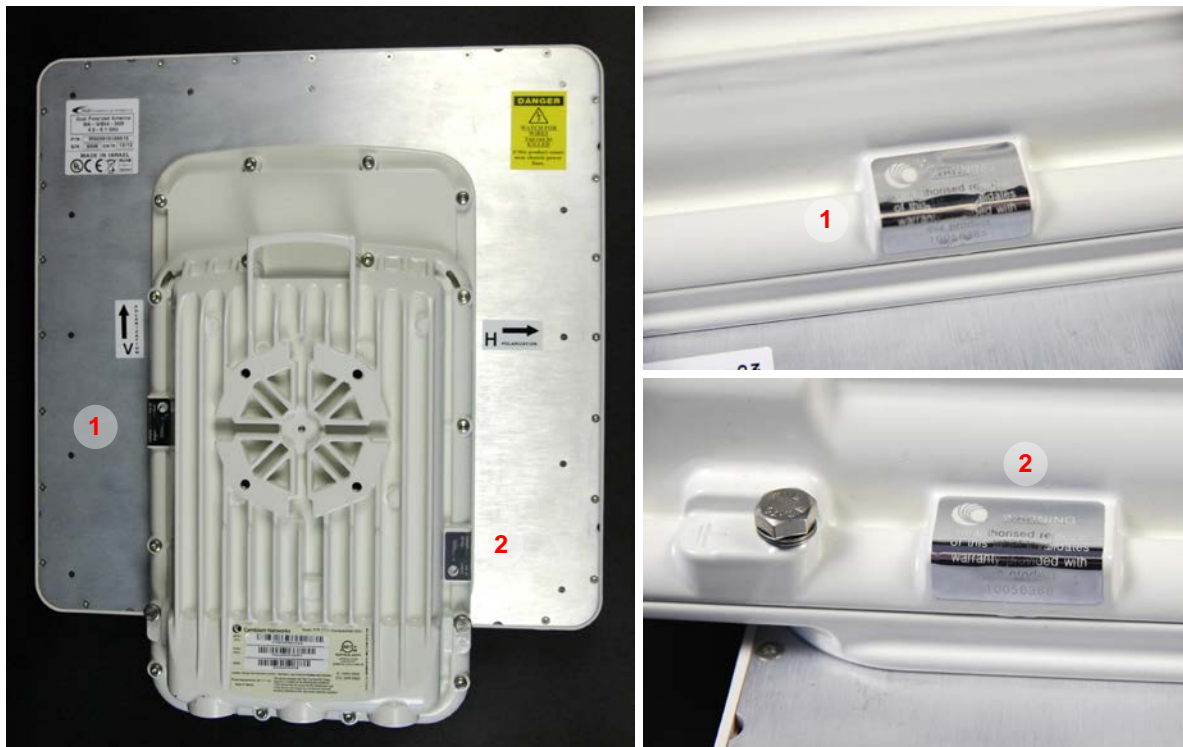
Figure 11 - Tamper-Evident Seal Locations on a White Connectorized+Integrated PTP 45700 Unit
