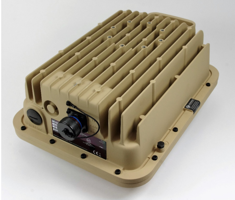
Figure 5 - PTP 78700 Connectorized Hardware Variant-Back and Front (Tan)
