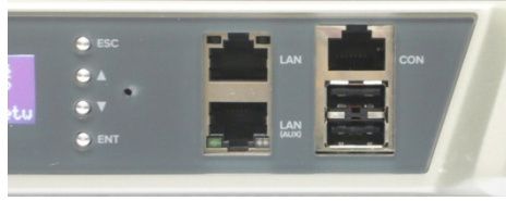
Figure 15 – CN9000 Series RJ45 Ethernet, Console and USB close-up
