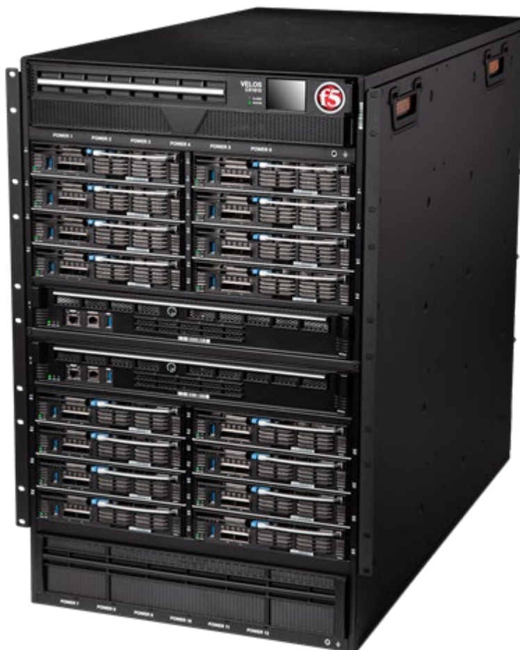
Figure 2: The F5 CX1610 Chassis, fully populated with 16 BX520 traffic blades
