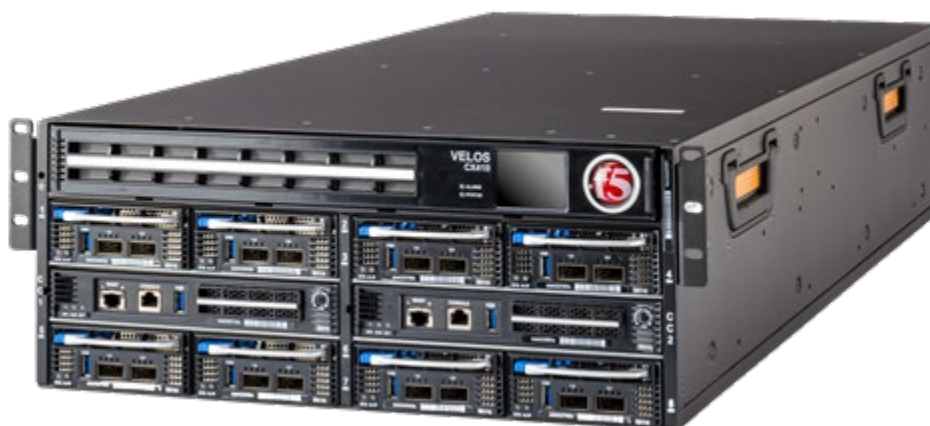
Figure 3: The F5 CX410 Chassis, fully populated with 8 BX110 traffic blades
