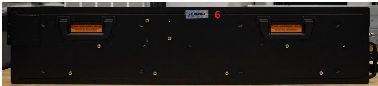
Figure 7: The right side of the module shows the placement of seal #6.
