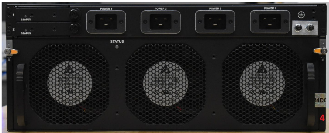
Figure 6: The rear side of the module shows the placement of seal #4, securing the fan unit to the chassis.
