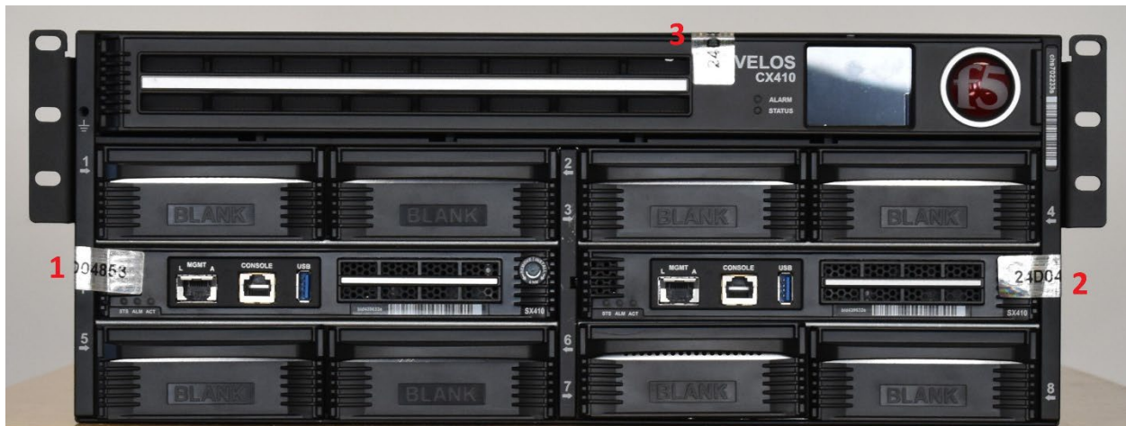
Figure 4: The front side of the module shows the placement of seals # 1, 2, and 3.
