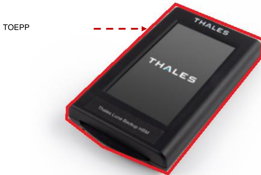
Figure 2-1: Thales Luna G7 Cryptographic Module HW 808-000064-005 and 808-000064-006
