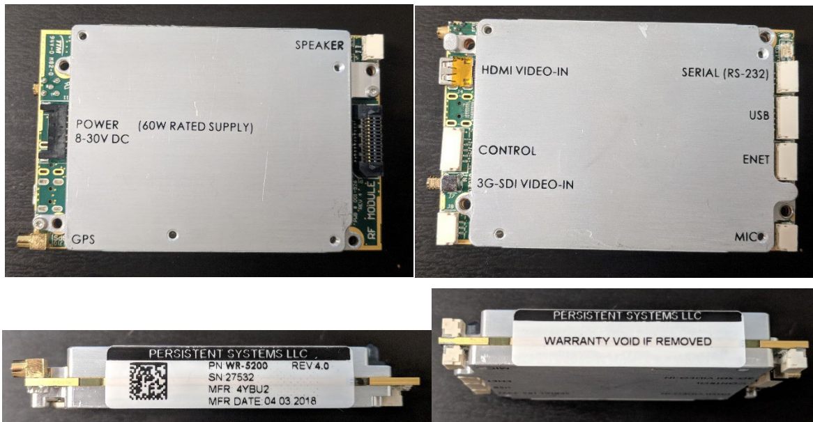
Figure 1 – Physical Boundary of Embedded Module
